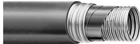
FLEXWELL Safety Pipe DN 25 - DN 100, except DN 40 with corrugated stainless steel primary pipe and corrugated steel outer containment pipe Worksheet FSR 1.03.02
