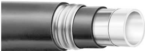
FLEXWELL Safety Pipe DN 20 - DN 150 with thermoplastic primary pipe and corrugated steel outer containment pipe (only on request) Consisting of a primary pipe, reinforcing bands, a corrugated outer containment pipe, a surveillance space, a double layer of BRUGG bitumen and a polyethylene jacket as external corrosion-proofing. Refer to the separate and special documentation covering technical details of this variant !
